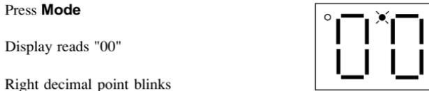
Use the **▲** and **▼** buttons to scroll to the password value (the factory default password is "25") and press the **Mode** button. Once the correct password value is entered, the display will read "01", which indicates that the PROGRAM mode has been accessed at the beginning of the parameter menu (01 is the first parameter), and the upper right decimal point will turn on solid. This is shown below:
